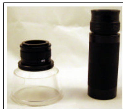
Macroscope after detachment showing magnifier on left and telescope on right.
